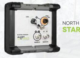
The NorthStar expands the capabilities of your RTK network over geographical obstructions, extending the range of the Resolute-Pin RTK Base.
